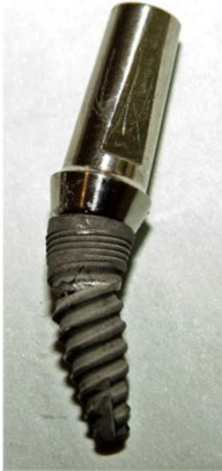
Fig. 7 Implant fracture after static fracture test
