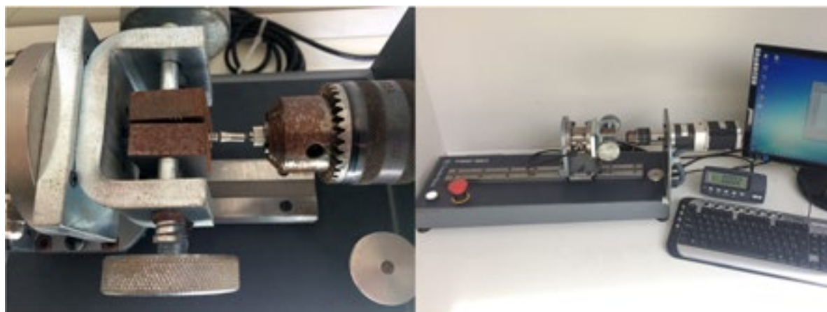
Fig. 5 a Scheme used in the torque test. b Torque machine
